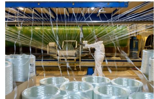
The station's mechanical strength, particularly its resistance to buckling, is achieved through a combination of orthogonal and helical filament winding.
